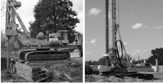
light-medium duty rig Watson 2000, crawler mounted capacity: 82 ft. depth, 5 ft. dia
