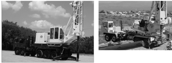
medium-heavy duty rig Watson 3000, carrier mounted up to 118 ft. deep, 7.9 ft. diameter torque: 136 kN-m crowd: 225 kN
