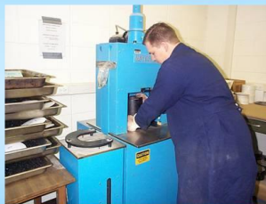
Compact the HMA plugs per KT-58
