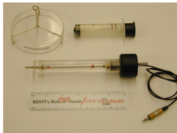
Figure 3 Petri dish, 20 ml syringe, and temperature sensor
