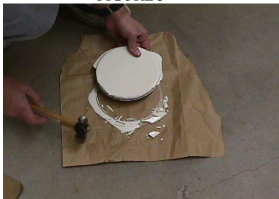
Removal of excess thermoplastic from lid
