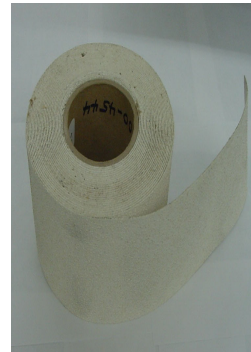
Roll of white, high durability pavement marking tape.
