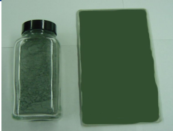
A bottle of organic powdered zinc primer beside a steel panel with applied zinc primer.
