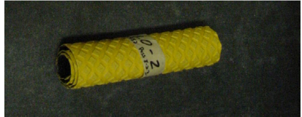
Yellow pavement marking tape that has been rolled and taped with masking tape.
