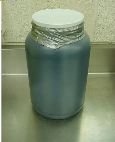
A gallon plastic container full of emulsified asphalt with the lid on and duct tape around the lid to help prevent any leaking.
