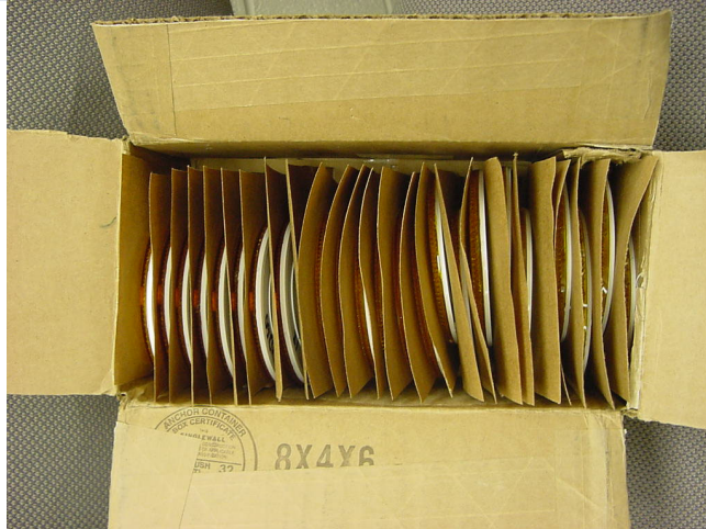
Center mount reflectors in a box with pieces of cardboard or cardstock between them and no space for movement.
