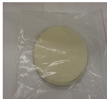
White thermoplastic applied to metal gallon can lid inside a clear plastic bag.
