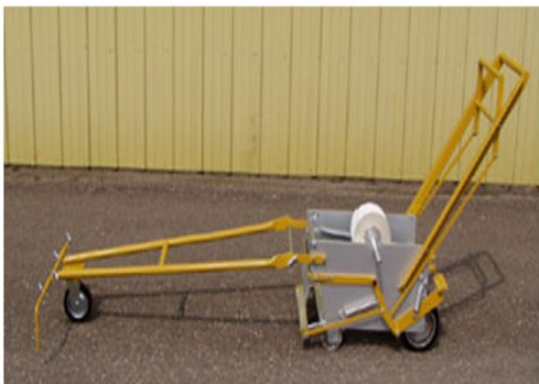
Three versions of pavement marking tape applicators. All variations of the same setup.
