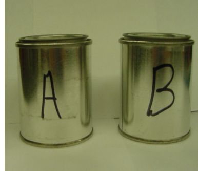
Two ½ pint paint cans. The left can is part A: the color component. The right can is part B: the hardener component.
