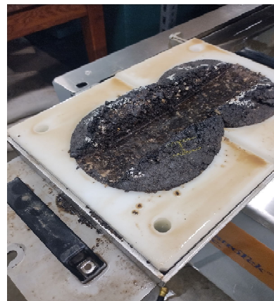
After 20,000 cycles or max depth in 50° C water
