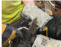
Cylinder with Sulfur cap
