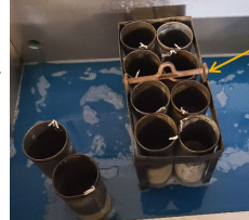
Aggregate Freeze and thaw cylinders in Glycol bath freezer
