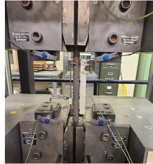
Tensile testing of Rebar
