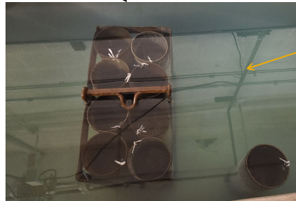
Aggregate Freeze and Thaw cylinders in water bath.
