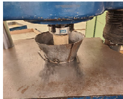
Cylinder being crushed with sulfur caps
