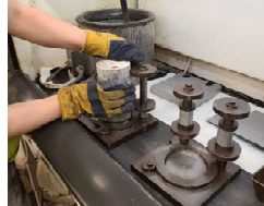
Cylinders being sulfur capped
