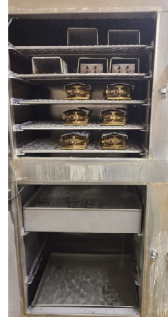
Curing environmental cabinet for cement cubes
