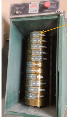
Aggregate Gradation sieve stack in Mary Ann gradation shaker.
