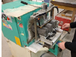
Cylinders being ground for sulfur capping
