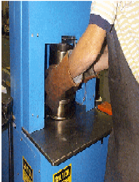
Placing Mold into the Compactor
