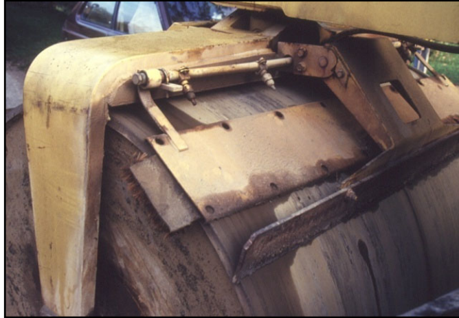
Spray nozzles not working properly
