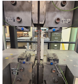
Tensile testing of Rebar
