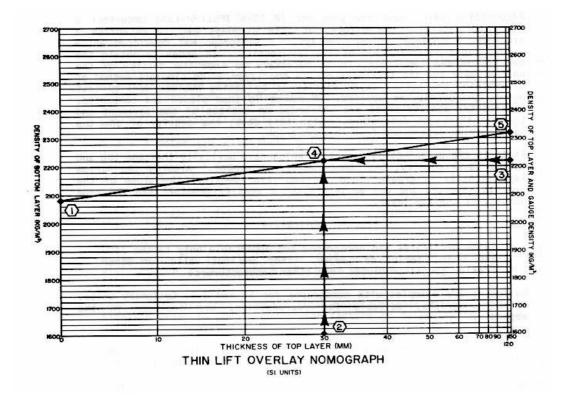
In this example, the bottom layer density (left scale) is 2080 kg/m³ with a mat of 30 mm thick overlaying it. A backscatter density test on the top of the mat (right scale) yielded a result of 2220 kg/m³. A line is then drawn from 2080 kg/m³ on the left scale through the intersection of 30 mm (bottom) and 2220 kg/m³ (right) and extended to the right. The correct density for the top layer is then read from the nomograph as  $2320 \text{ kg/m}^3$  on the right scale.
